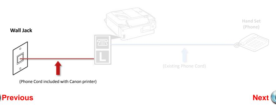
• Plug the provided phone cord into the "L" jack located on the rear of the multifunction
